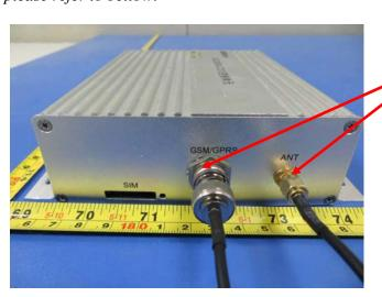
The Antenna was fixed permanently by special glue (AB Glue)
