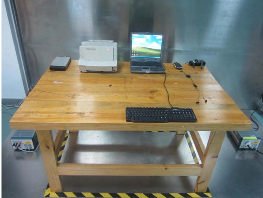
Conducted Emission - Front View
