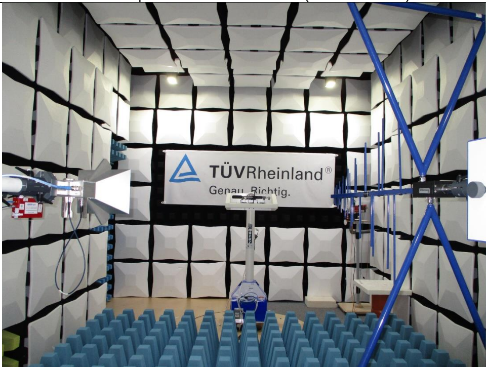
Test Setup: Radiated Measurements (1 GHz to 40 GHz)
