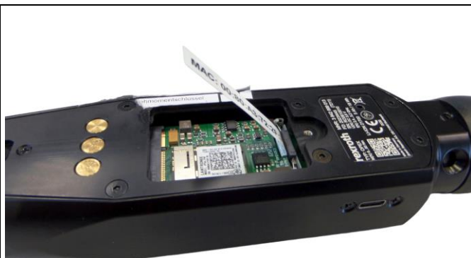
Picture 5 :Radio Module location image & Antenna Location
