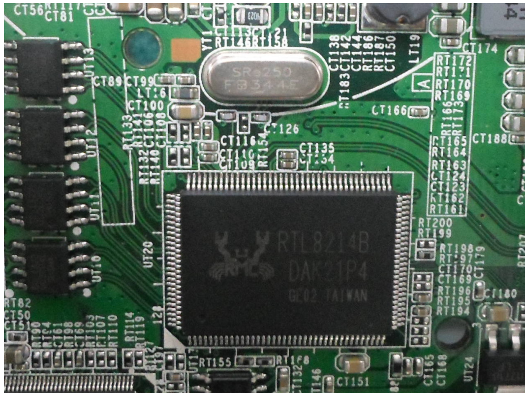
FIGURE 9 GPON SFU (M/N: 7269G) CHIP AND CRYSTAL #1 ON MAIN BOARD
