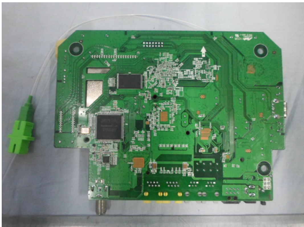
FIGURE 8 GPON SFU (M/N: 7269G) MAIN BOARD (SOLDERED SIDE)
