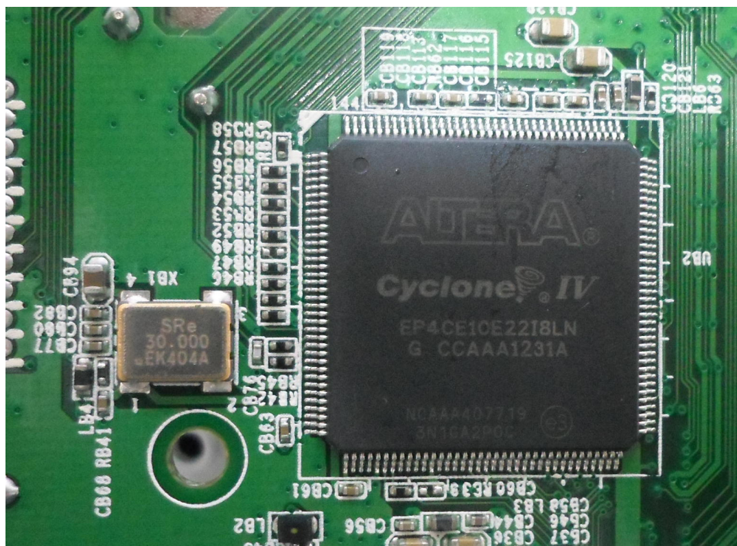
FIGURE 10 GPON SFU (M/N: 7269G) CHIP AND CRYSTAL #2 ON MAIN BOARD
