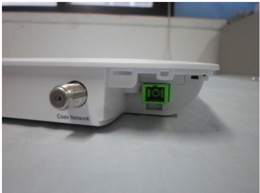
FIGURE 4 GPON SFU (M/N: 7269G) PORT #2
