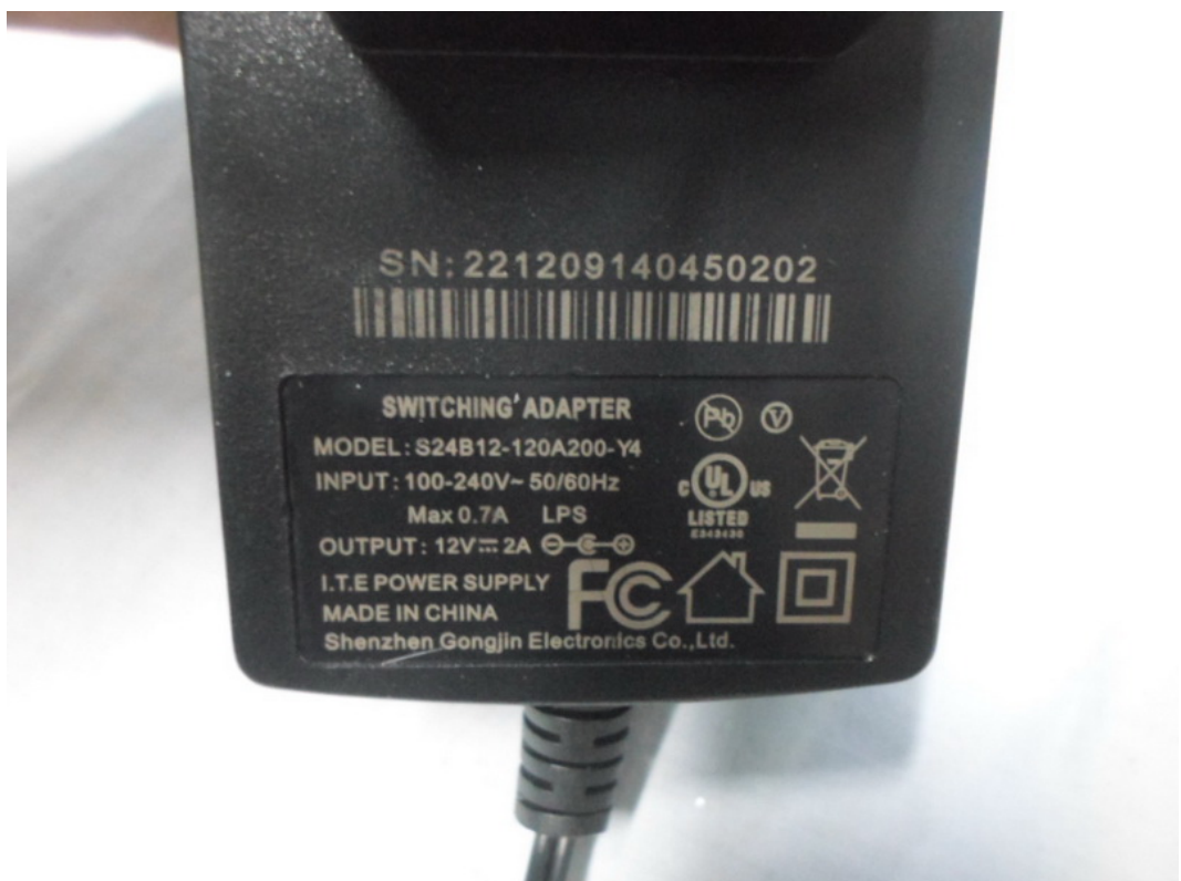
FIGURE 16 GPON SFU (M/N: 7269G) ADAPTER (LABEL)
