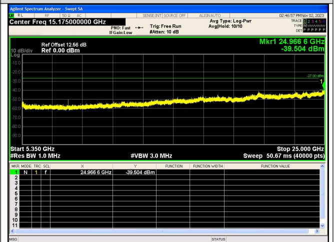
Spurious Emission:5350~25000.0 MHz IEEE 802.11ac_Channel 42_80MHz_Antenna 0
