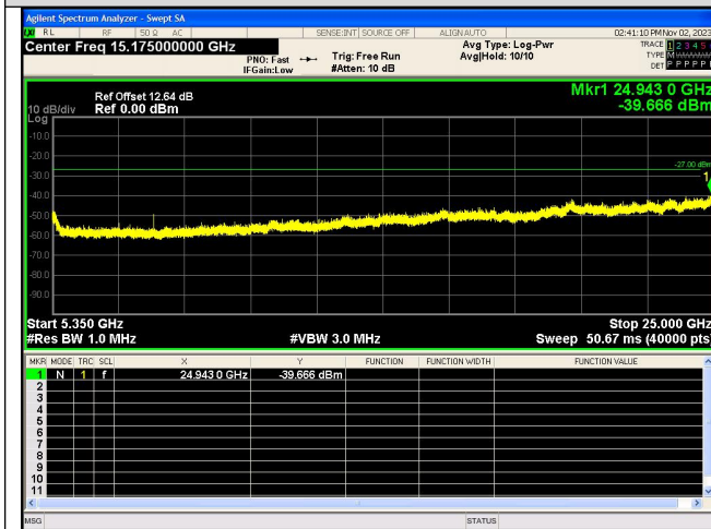
Spurious Emission:5350~25000.0 MHz IEEE 802.11ac_Channel 46_40MHz_Antenna 0
