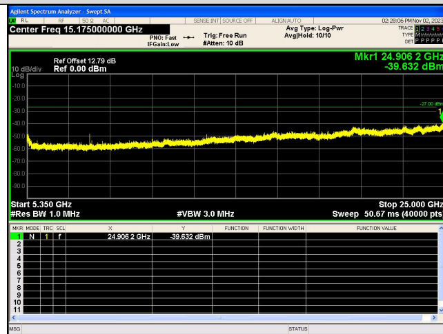
Spurious Emission:5350~25000.0 MHz IEEE 802.11n_Channel 38_40MHz_Antenna 0
