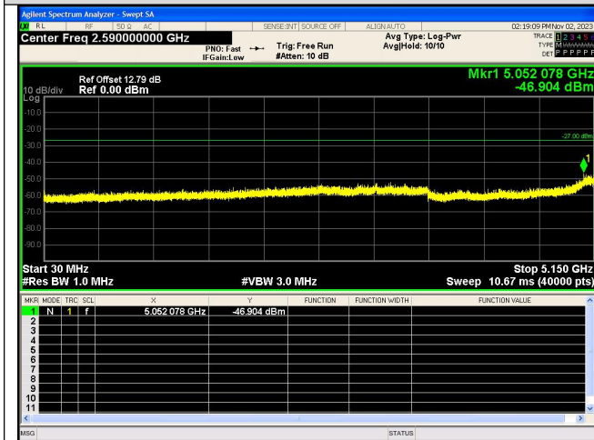
Spurious Emission:30.0~5150 MHz IEEE 802.11ac_Channel 40_20MHz_Antenna 0
