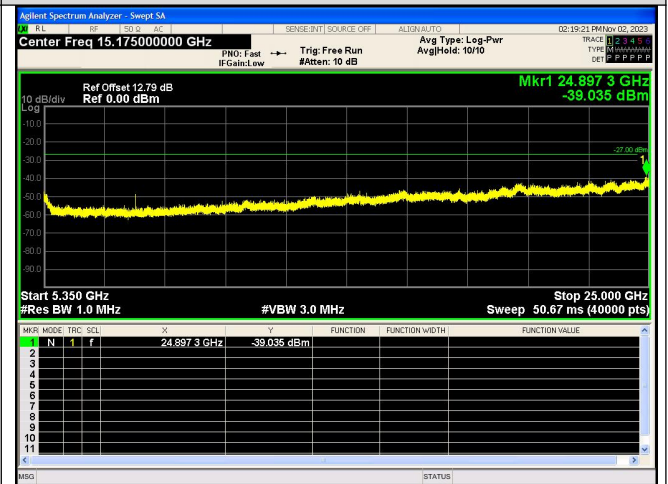
Spurious Emission:5350~25000.0 MHz IEEE 802.11ac_Channel 40_20MHz_Antenna 0
