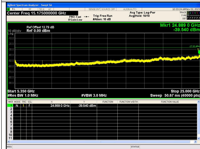
Spurious Emission:5350~25000.0 MHz IEEE 802.11ac_Channel 36_20MHz_Antenna 0
