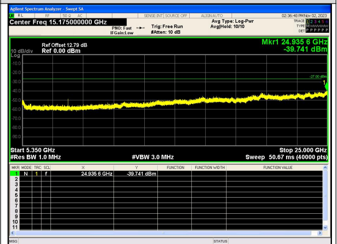
Spurious Emission:5350~25000.0 MHz IEEE 802.11ac_Channel 38_40MHz_Antenna 0
