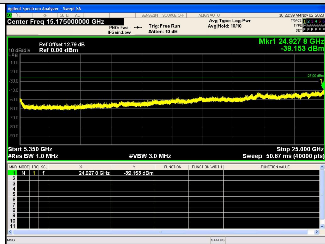
Spurious Emission:5350~25000.0 MHz IEEE 802.11n_Channel 40_20MHz_Antenna 0
