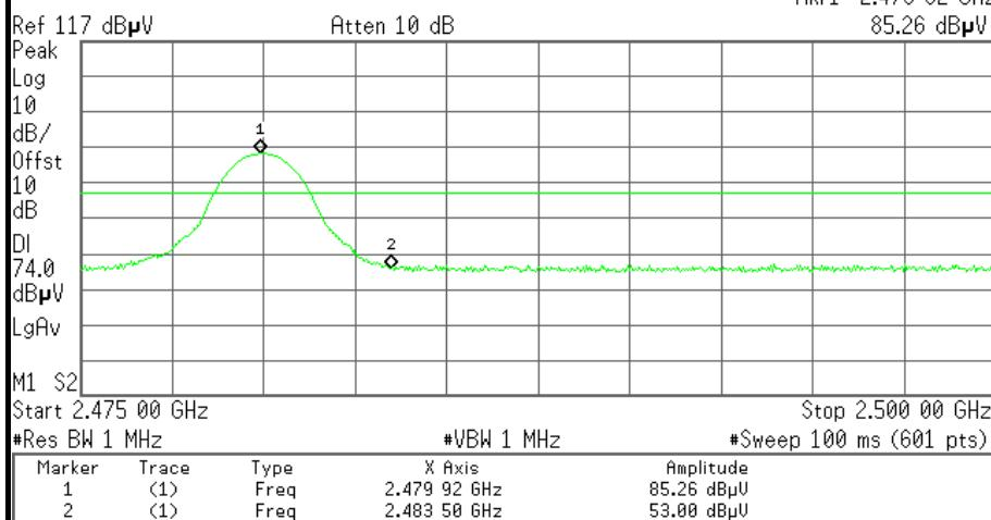
**Detector mode : Average****Polarity : Vertical****CH High / 8-DPSK**
