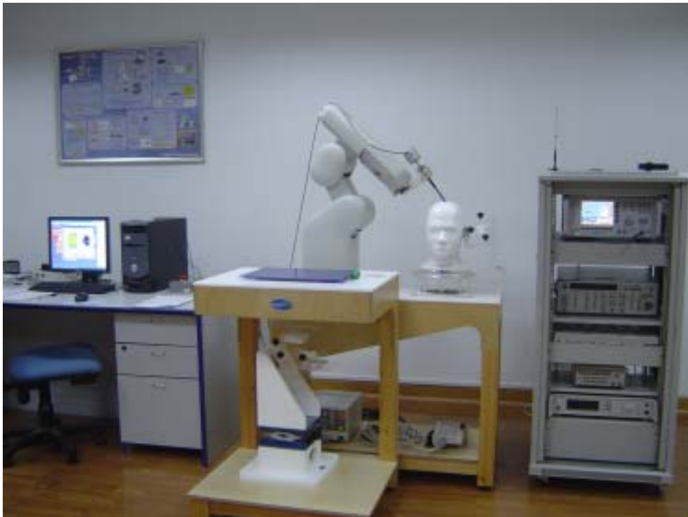
Fig.1 SARA2 System Test Layout
