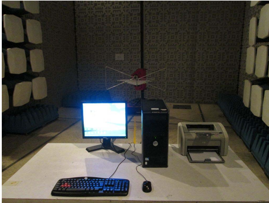
RADIATED EMISSION TEST SETUP-1
