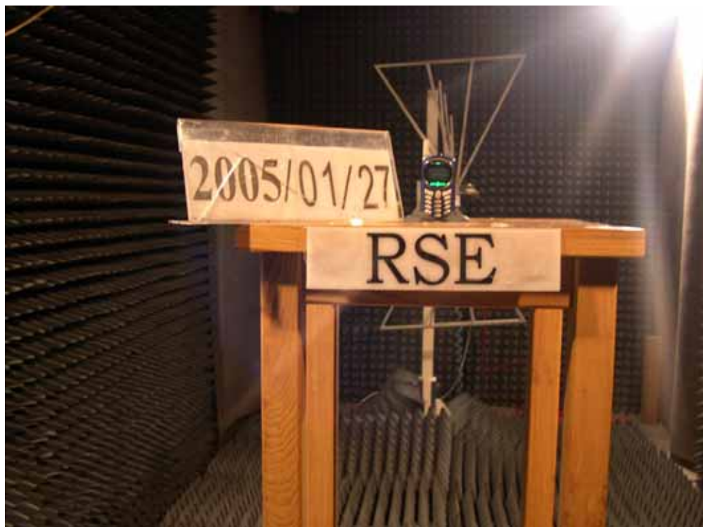
TCL558 Radiated Spurious Emission Test Setup
