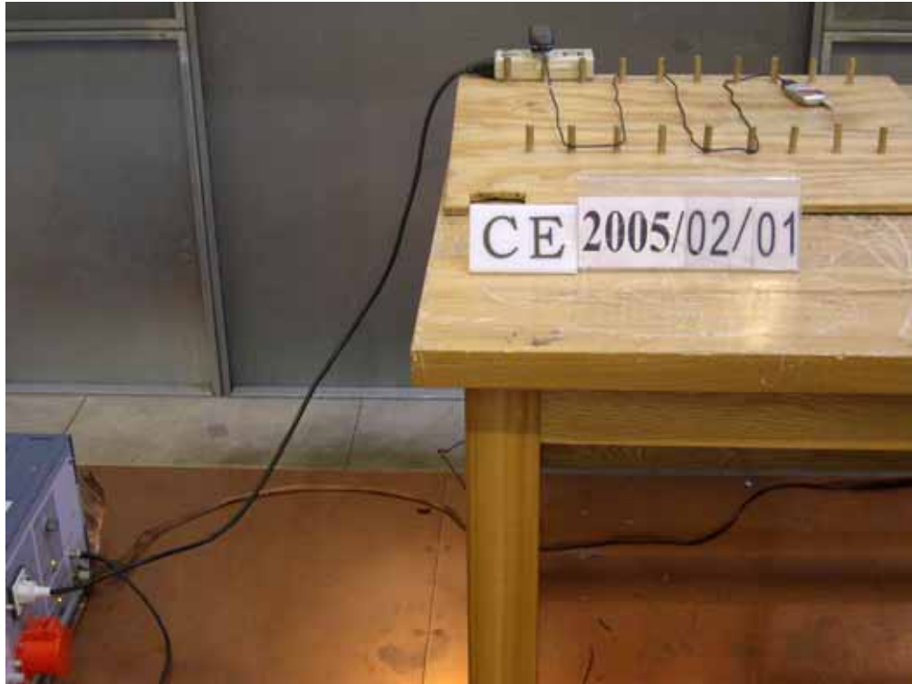
TCL538 Conducted Emission Test Setup
