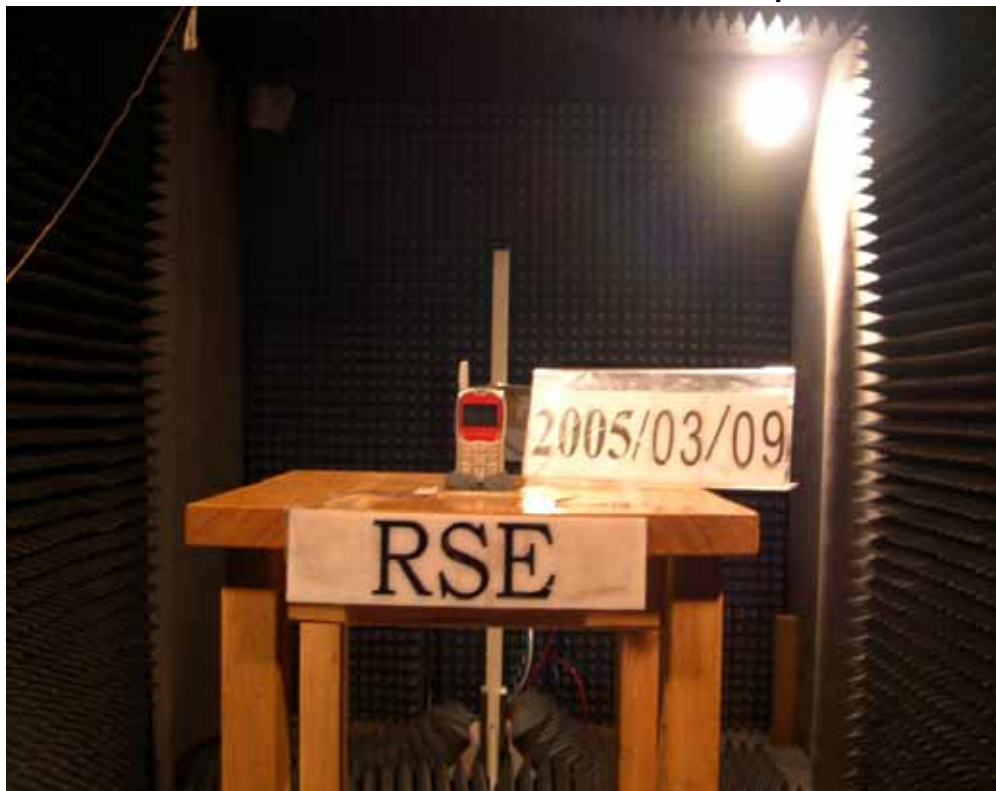
TCL538 Radiated Spurious Emission Test Setup
