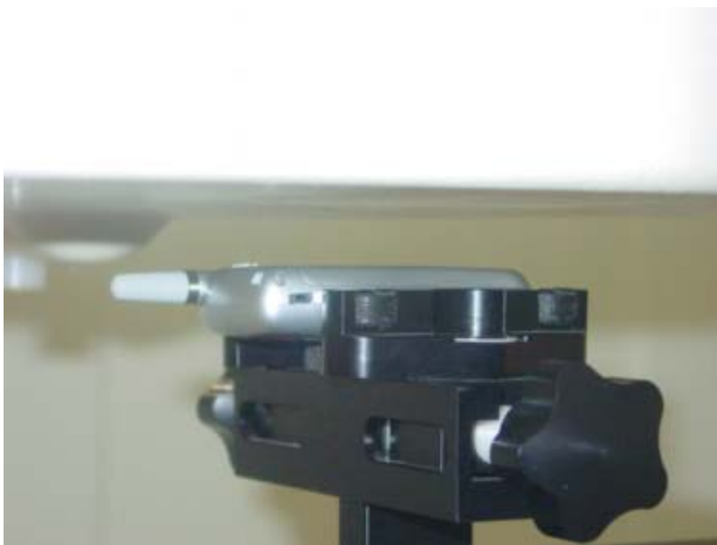
Picture 6 Flat Phantom -- Body-worn Position (toward phantom, the distance from handset to the bottom of the Phantom is 1.5cm)
