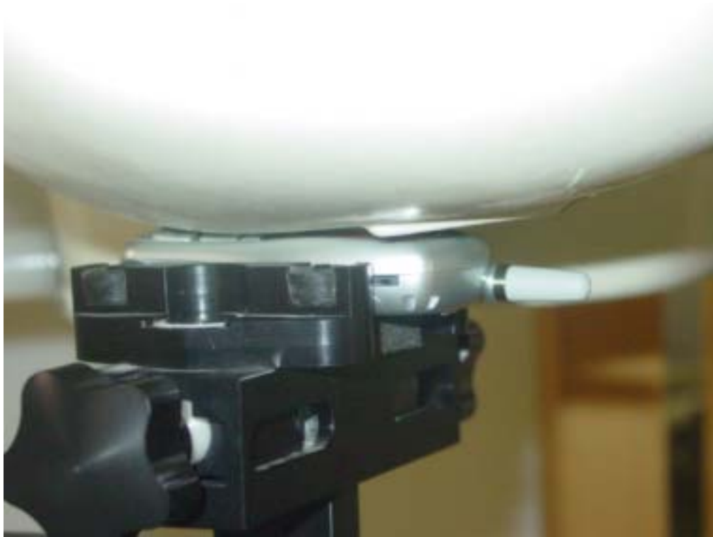
Picture 2 Left Hand Touch Cheek Position
