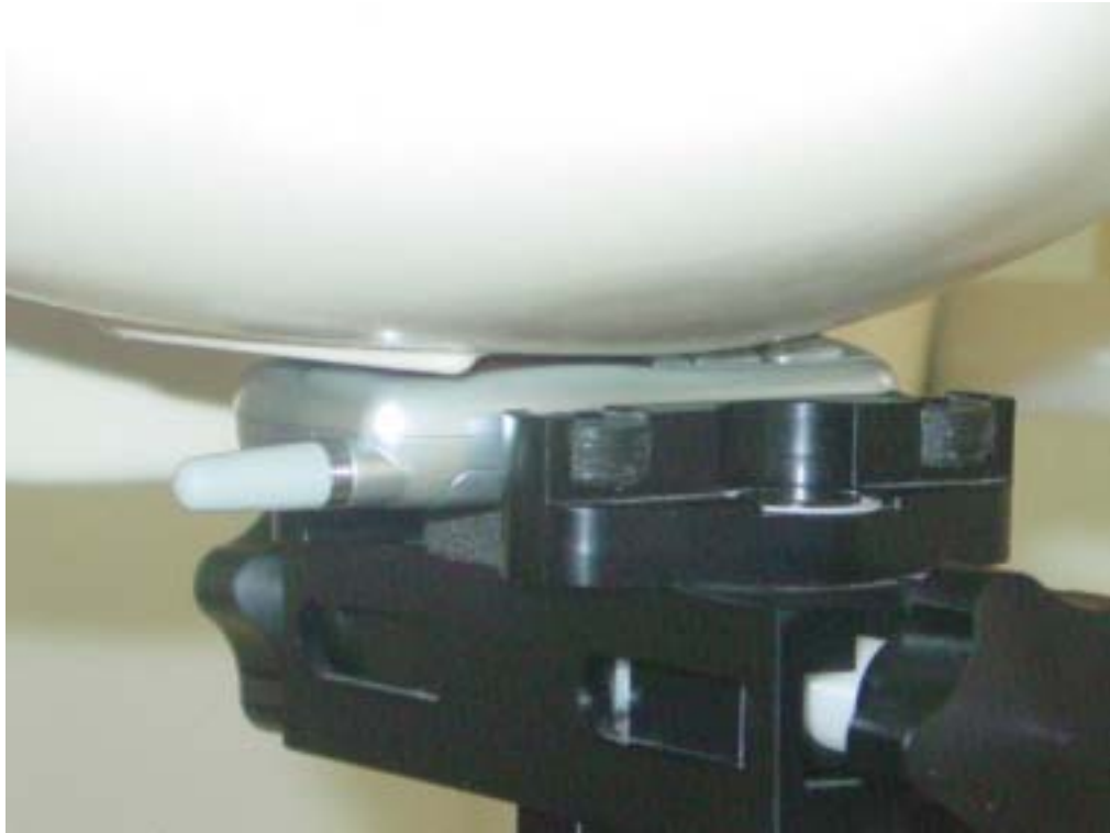
Picture 4 Right Hand Touch Cheek Position
