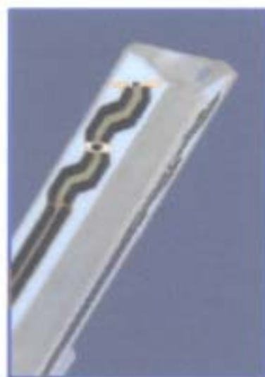
Figure 3. ET3DV6 E-field Probe
