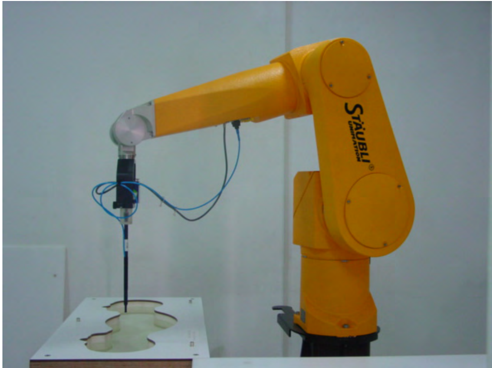
Picture 1 Specific Absorption Rate Test Layout
