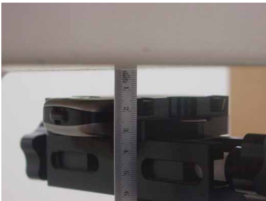
Picture 7 Flat Phantom -- Body-worn Position (towards phantom, the distance from handset to the bottom of the Phantom is 1.5cm)
