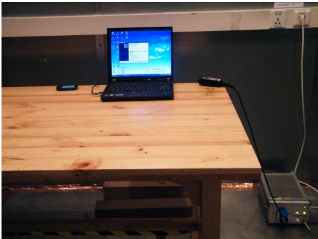
Picture 3 Conducted Emission Test Setup
