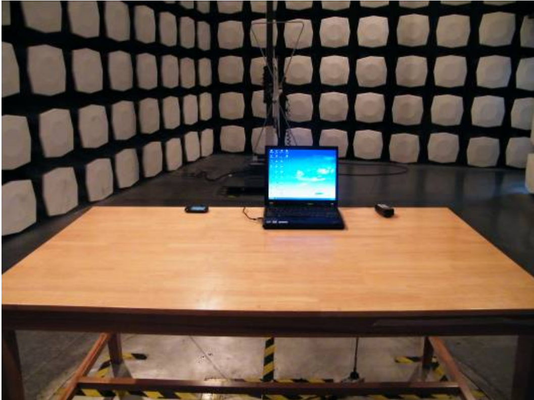
Picture 2 Radiated Emission Test Setup
