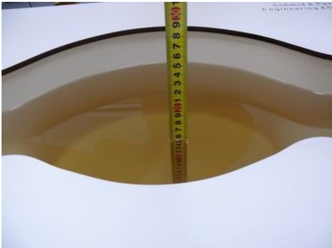
Picture 3: Liquid depth in the Flat Phantom (835 MHz, 15.4cm depth)
