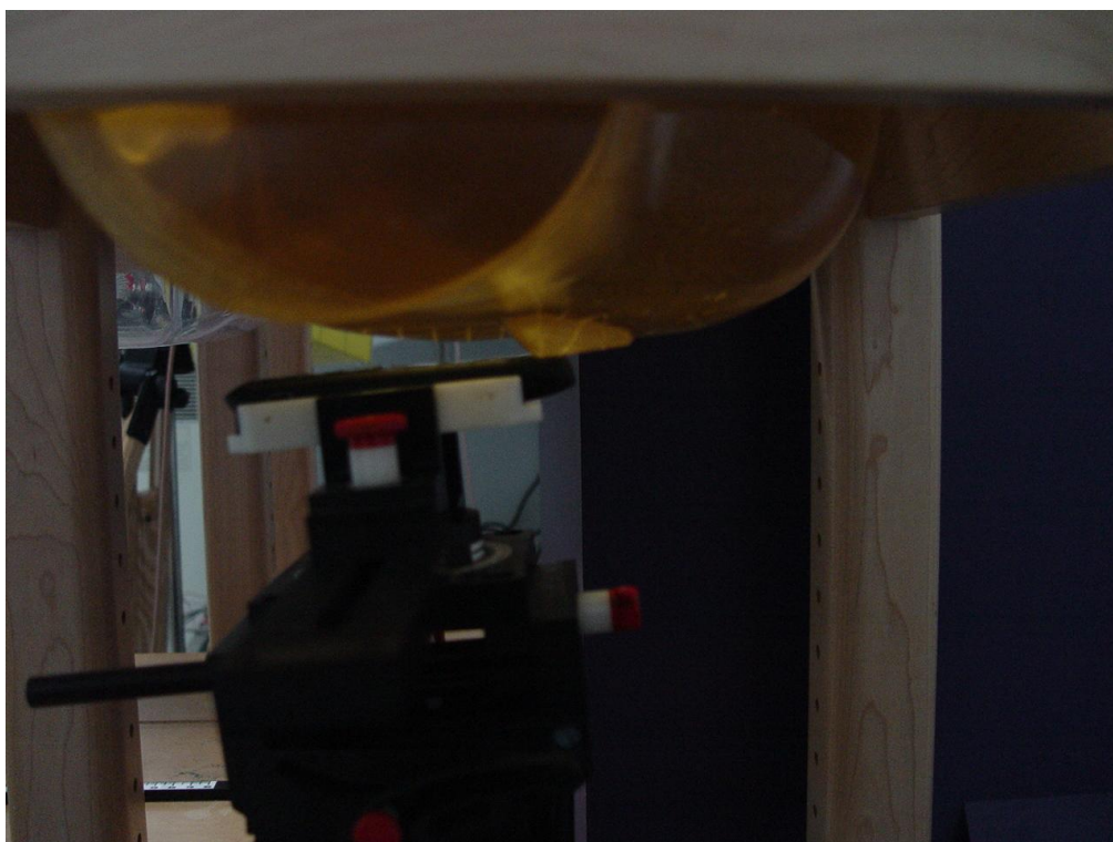
Figure B.4 EUT Right Cheek Position
