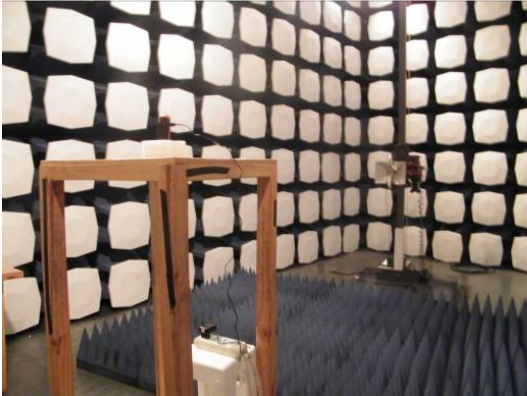
Picture 2: Radiated Spurious Emissions Test setup
