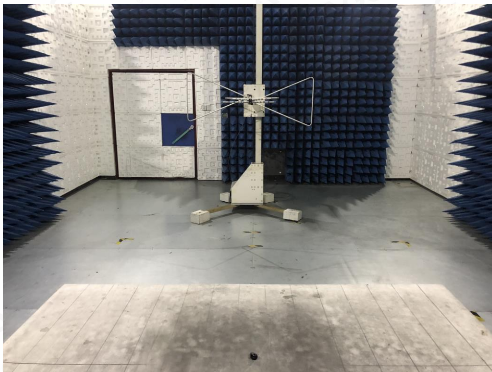
RADIATED EMISSION TEST SETUP ABOVE 1GHZ
