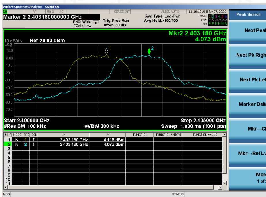
TEST PLOT FOR FREQUENCY SEPARATION
