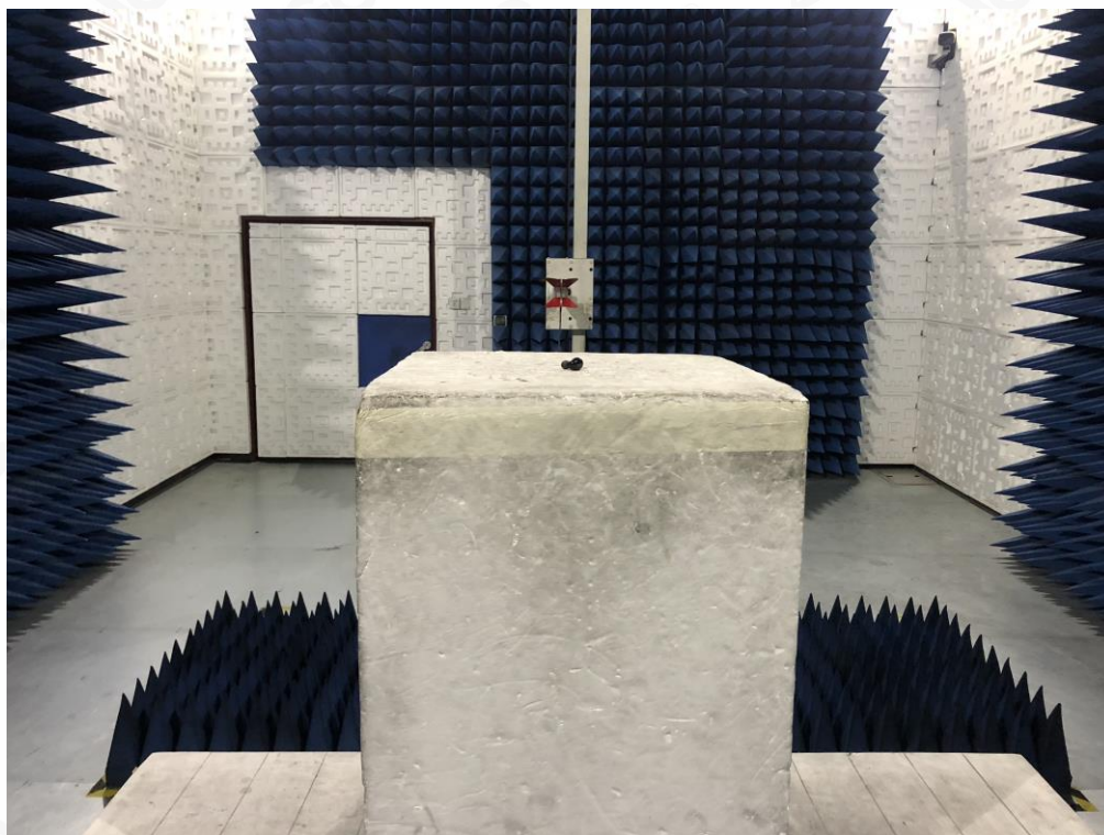
RADIATED EMISSION TEST SETUP ABOVE 1GHZ
