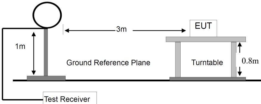
For Radiated Emission 30-1000MHz
