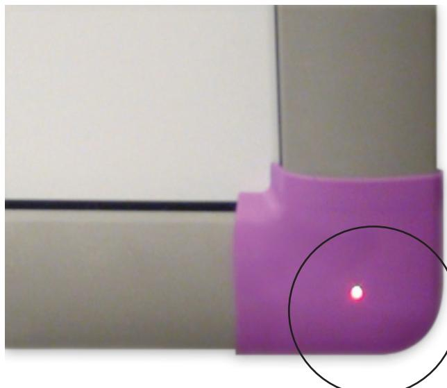
A red light located at the bottom right corner of the board indicates that the board is receiving power through the USB cable. A blue light indicates proximity of the pen to the board. See picture for indicator light location.
