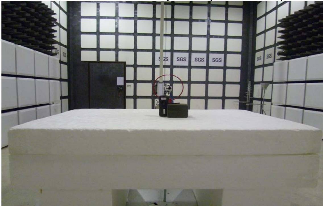
**Radiated Emission Set up Photo (Below 1GHz)**
