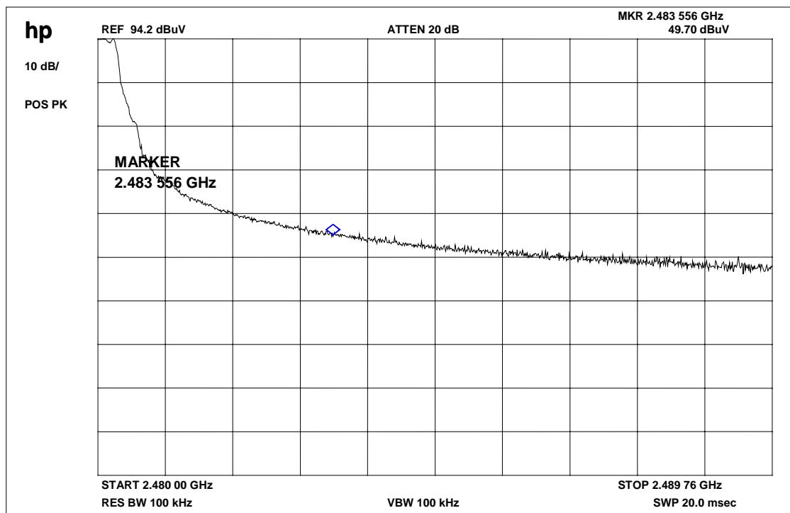
**Marker-Delta-Value : 44.5 dB****This measurement was made to show that the behavior of the system is conform to****FCC 15.205 (restricted bands)****REFERENCE NUMBER(S) OF TEST EQUIPMENT USED****(for reference numbers see test equipment listing)****17 – 24, 64**
