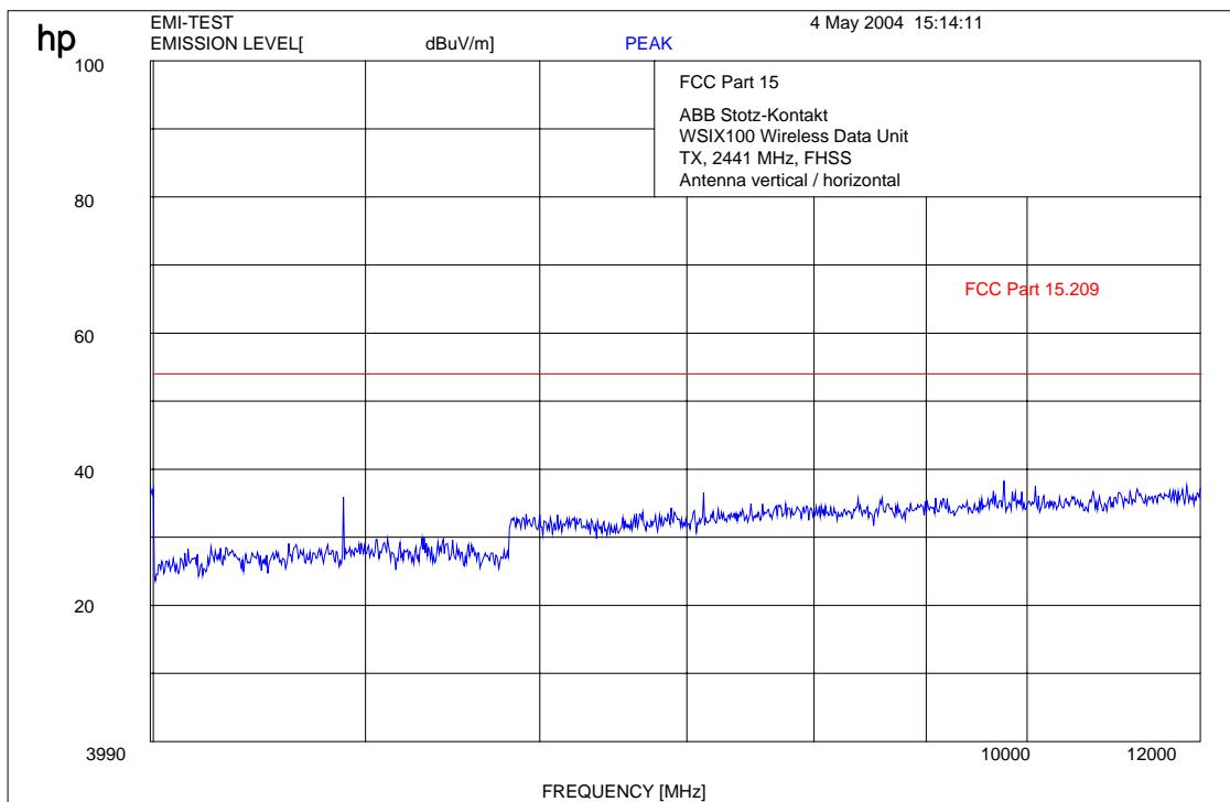
**$f < 1 \text{ GHz}$  : RBW/VBW: 100 kHz** **$f \geq 1 \text{ GHz}$  : RBW/VBW: 1 MHz****LIMITS****SUBCLAUSE § 15.247 (c)**
