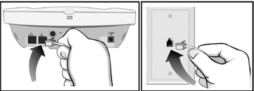
Figure 6. Connecting Prodigy to Your Phone Jack
