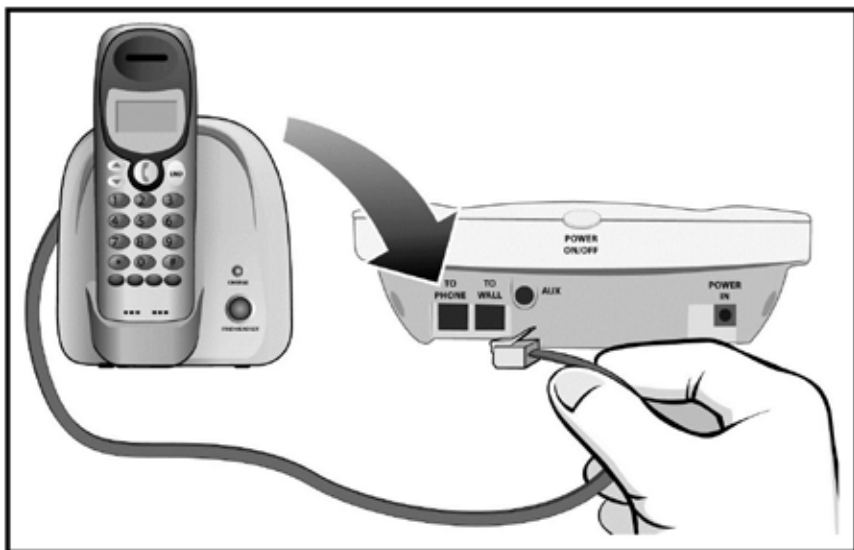
Figure 7. Connecting Your Home Telephone to Prodigy
