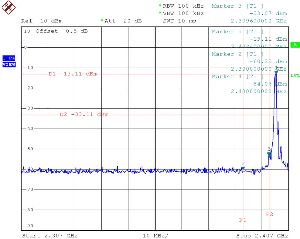
**Bluetooth/1 Mbps/The max. radio frequency power in any 100 kHz bandwidth within the frequency band**
