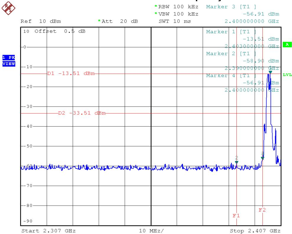
**Bluetooth/3 Mbps/The max. radio frequency power in any 100 kHz bandwidth within the frequency band**
