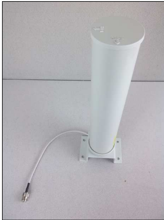
Figure 4: External Photo – Yagi Antenna
