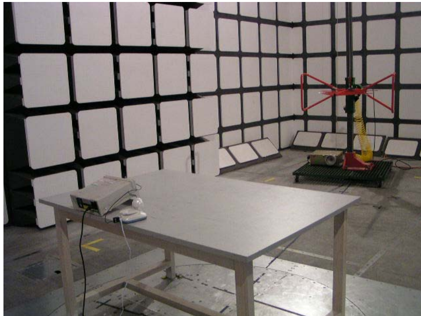
30 MHz – 1000 MHz: Radiated Emission - Rear View
