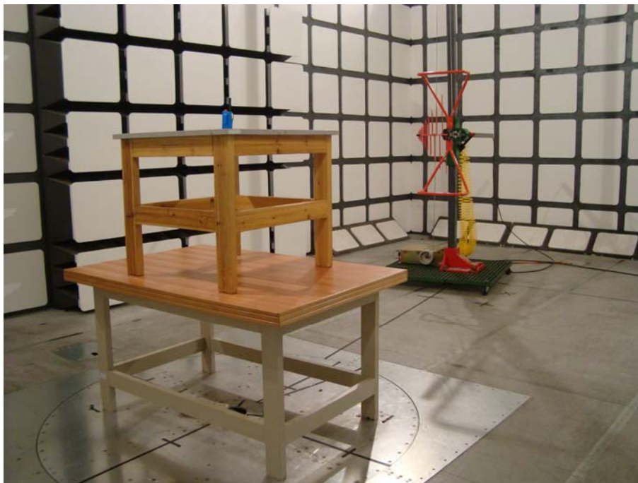
Radiated Emission - Rear View (Above 1GHz)
