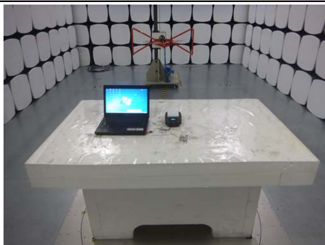
Radiated Spurious Emissions Test Setup Below 1GHz
