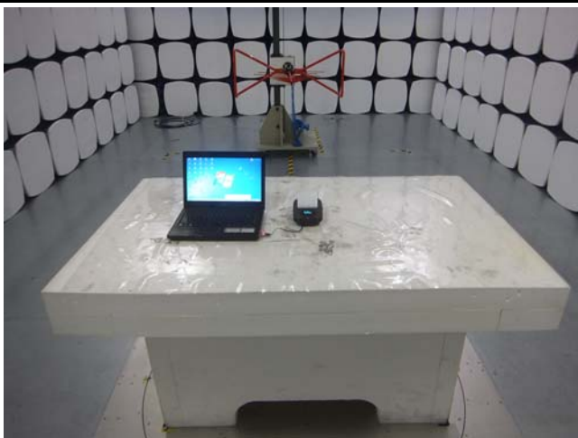
Radiated Spurious Emissions Test Setup Below 1GHz
