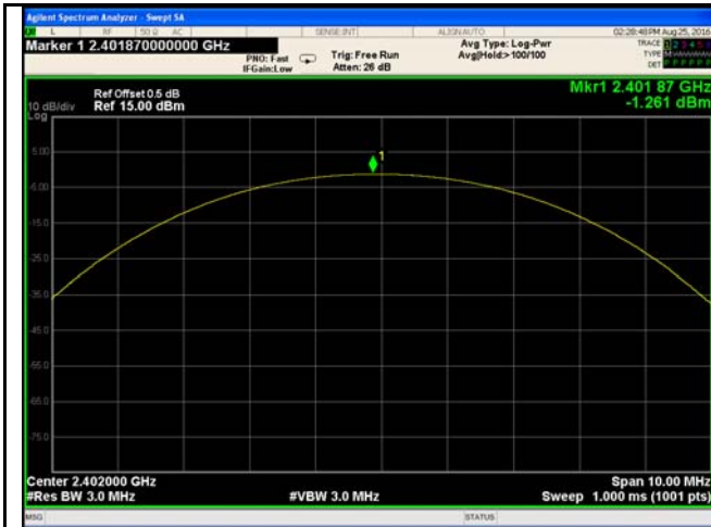
8DPSK Output power - Low CH 2402
