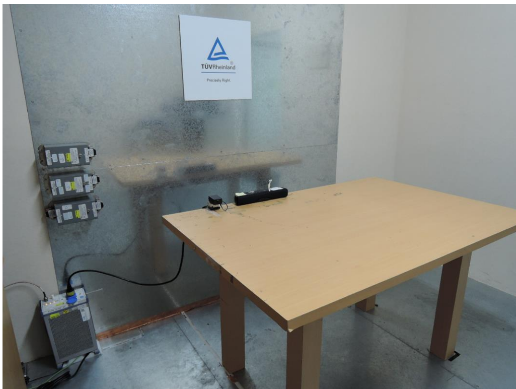
Photograph 6: Set-up for for Mains Conducted testing Front
