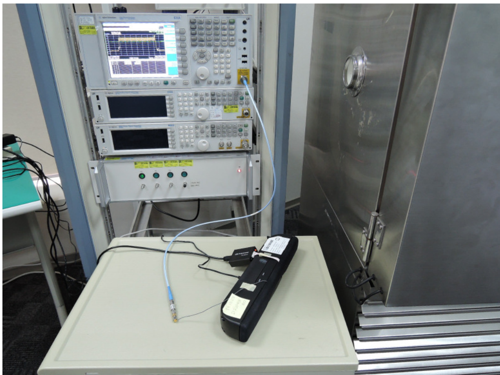
Photograph 4: Set-up for Conducted testing
