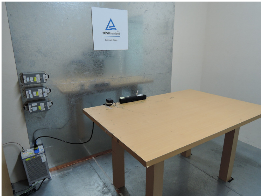
Photograph 6: Set-up for for Mains Conducted testing Front
