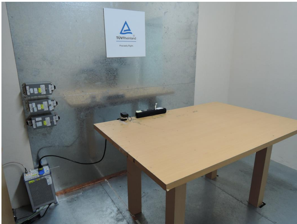
Photograph 6: Set-up for for Mains Conducted testing Front
