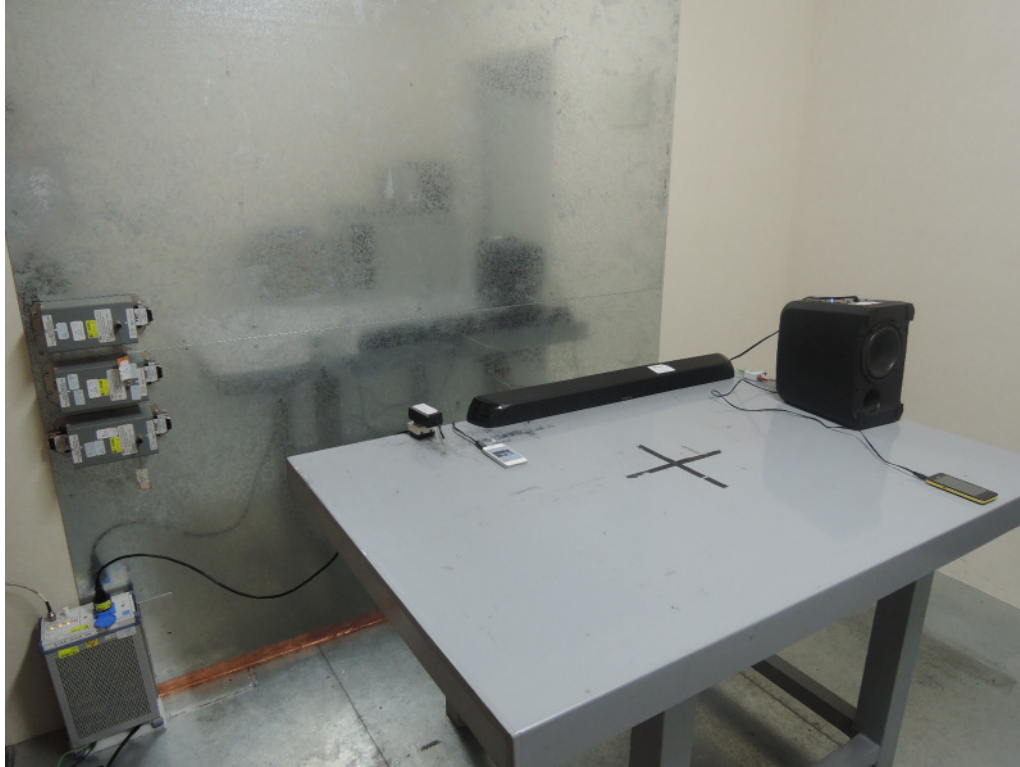
Photograph 6: Set-up for for Mains Conducted testing Front
