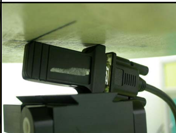
D. The edge (left) of the EUT face to the phantom with 0mm-separation distance.
