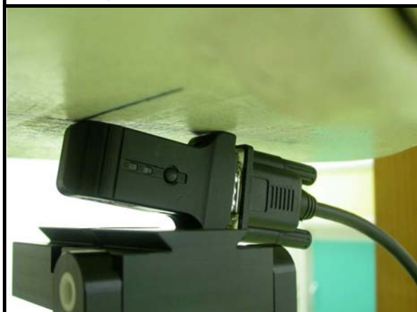
C. The edge (right) of the EUT face to the phantom with 0mm-separation distance.
