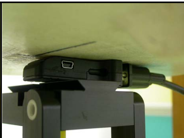
B. The front of the EUT face to the phantom with 0mm-separation distance.
