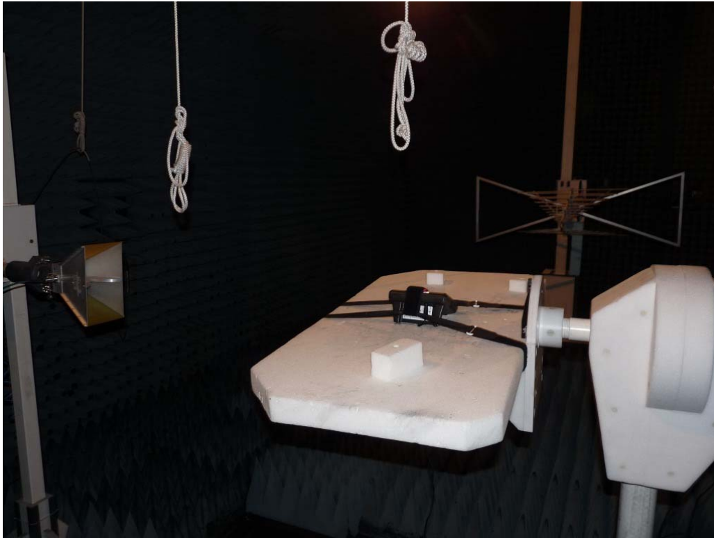
Photo 1: (Part 24/22) Test setup for radiated measurements
