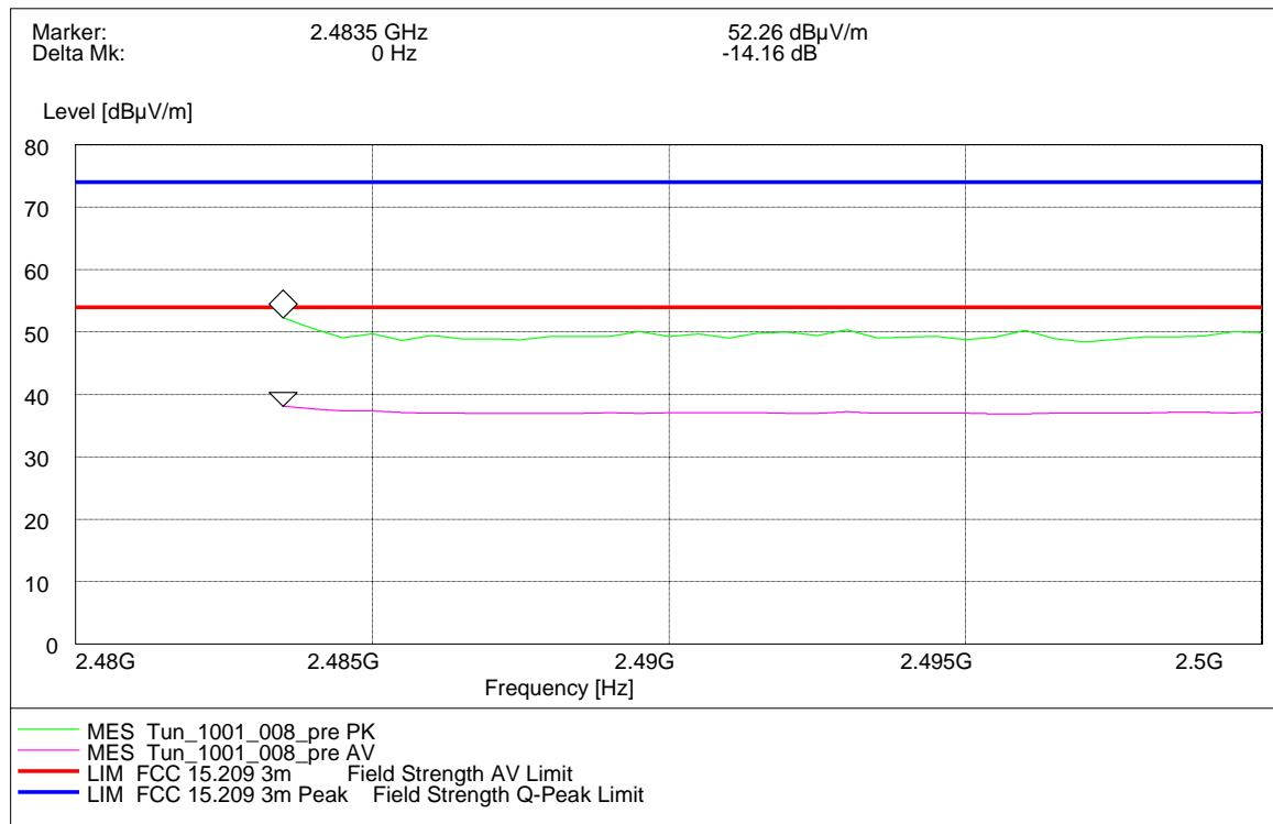
Radiated measurement (higher band edge)
