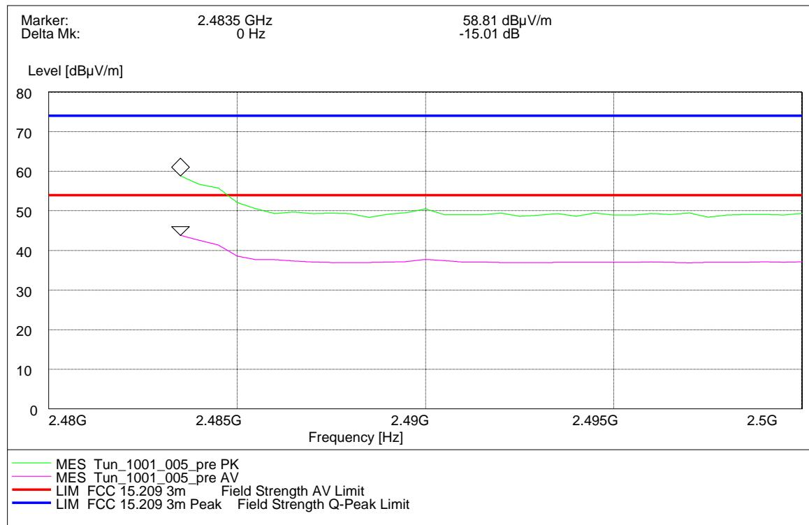
Radiated measurement (higher band edge)
