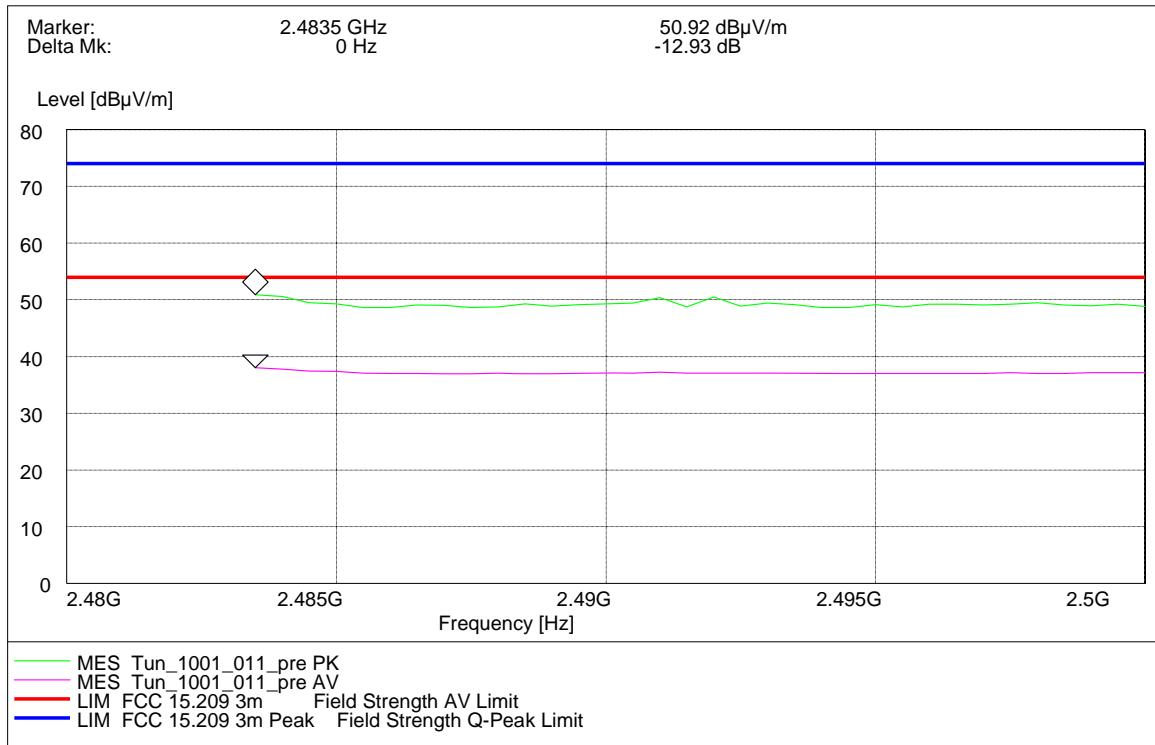
Radiated measurement (higher band edge)
