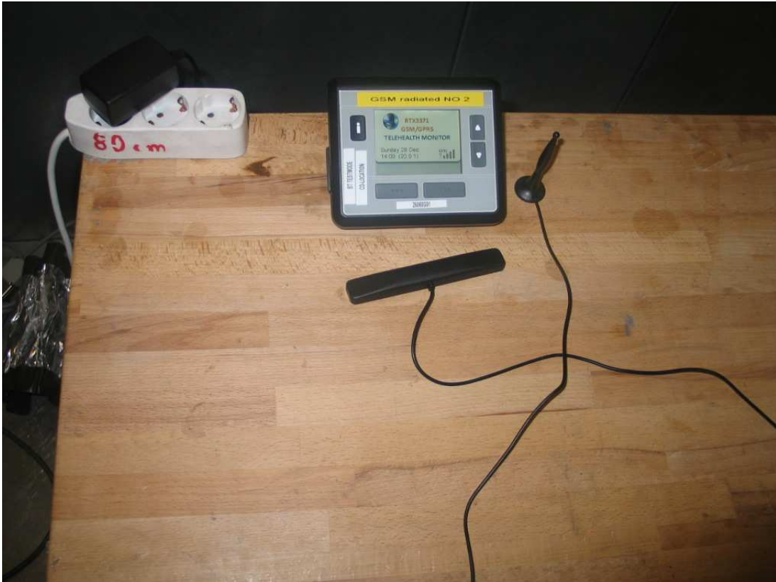
Photo 5: Test setup for the test AC mains conducted
