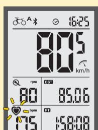
For your safety, PanoComputer has a Max Heart Rate Alarm function. When Heart Rate exceed Max limit, the Heart icon will be shown in black. Set Max Heart Rate limit in Topeak PanoBike App.
