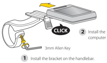
1 Install the bracket on the handlebar.
