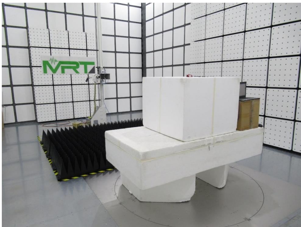
**Description: Radiated Emission Test Setup**
