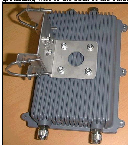
Figure 2-16 Attach the Mounting Bracket to Outdoor Unit
