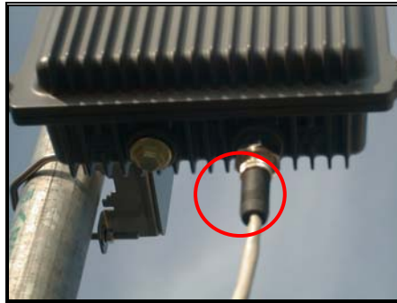
Figure 2-19 Connect Cat-5 cable to the outdoor unit
