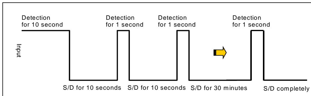
The embedded detector of repeater is designed to detect whether the RF output power of the repeater exceeds a prescribe limit on the downlink or uplink. If it catches some overpowers during 10 seconds and more, the repeater itself shutdown automatically.
