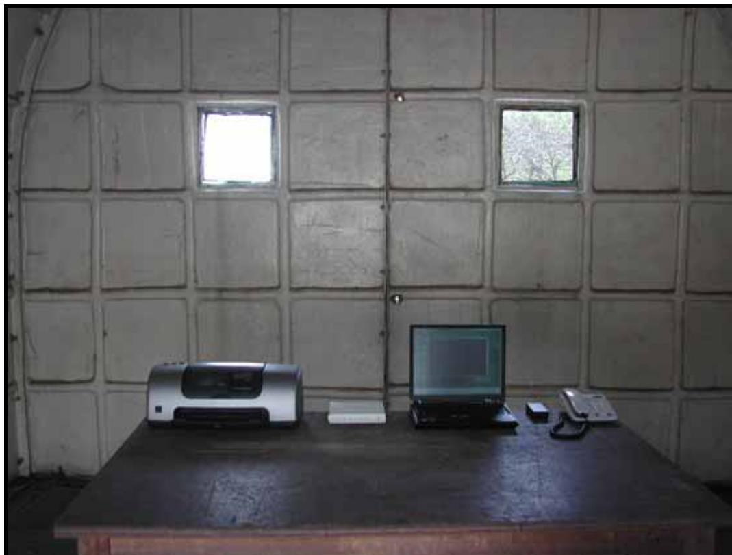
Photograph 2: Setup for Radiated Emissions
