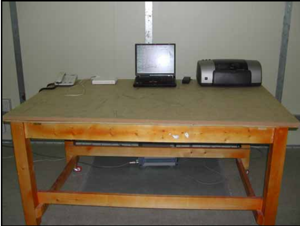
Photograph 1: Setup for Conducted Emissions
