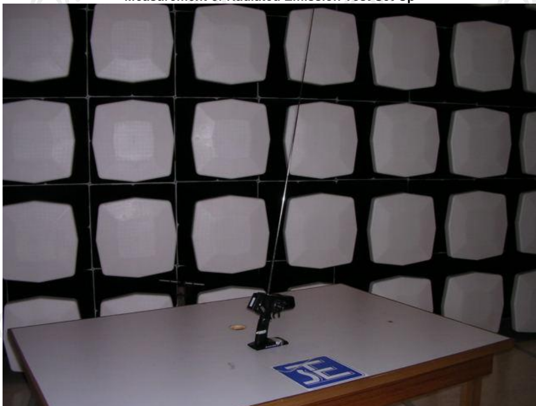
Measurement of Radiated Emission Test Set Up
