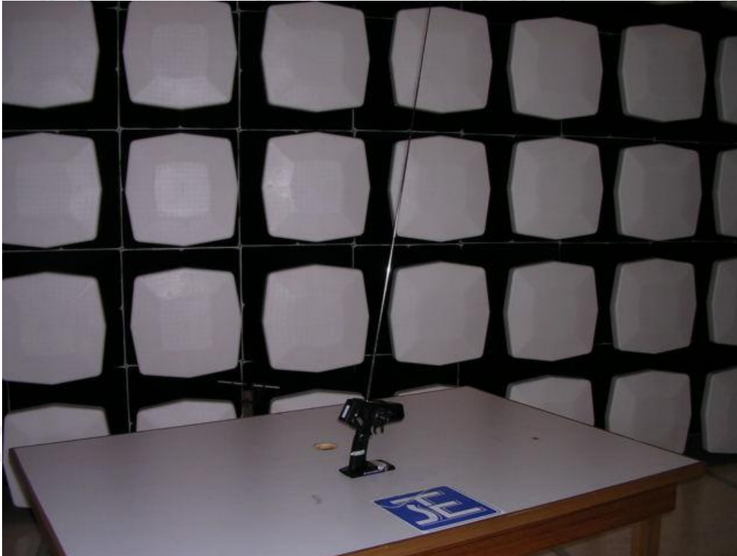
Measurement of Radiated Emission Test Set Up
