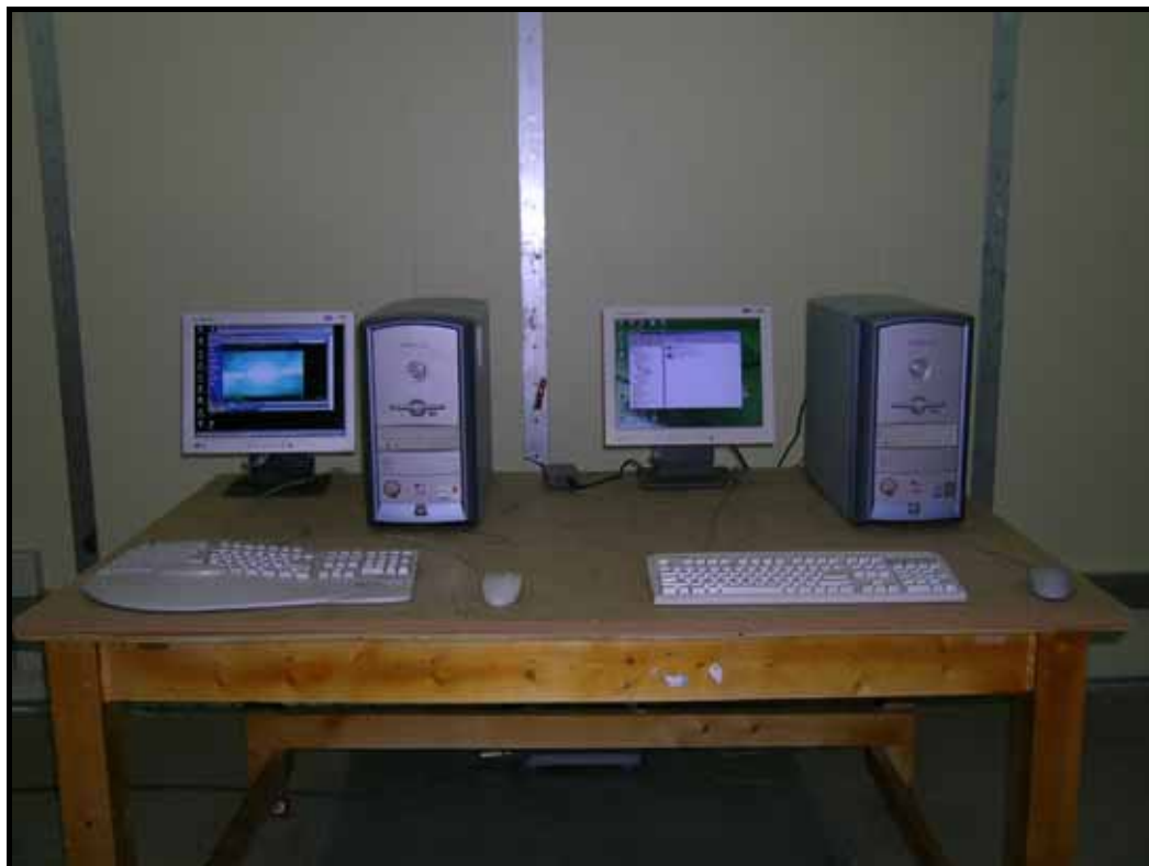
Photograph 1: Setup for Conducted Emissions
