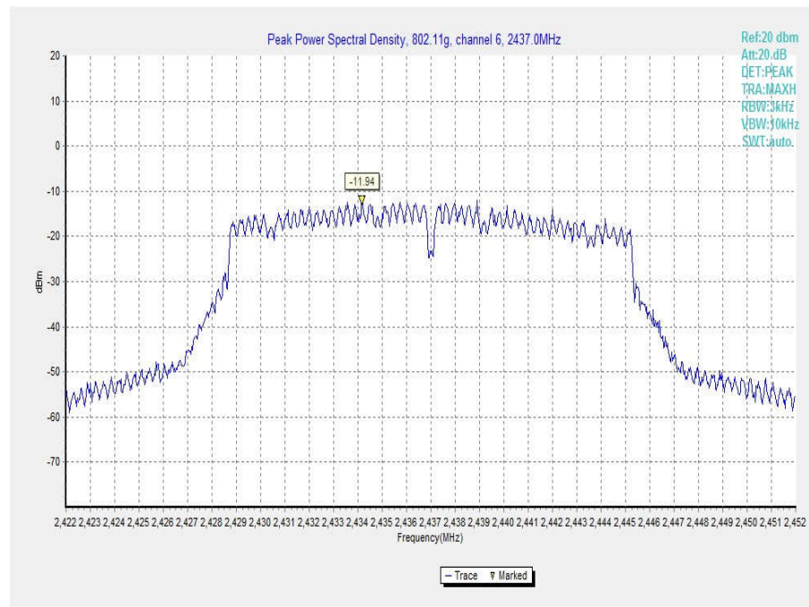
Fig.89 Power Spectral Density (802.11g, Ch 6)
